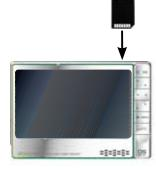
The memory card slot, located on top of the device, on the right side, allows you to insert one of the following cards (which are not supplied):
